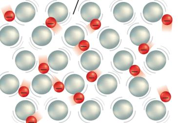
In metals, electrons can move freely. When thermal energy is added, no strong bonds have to be broken before the electrons can start moving faster.
